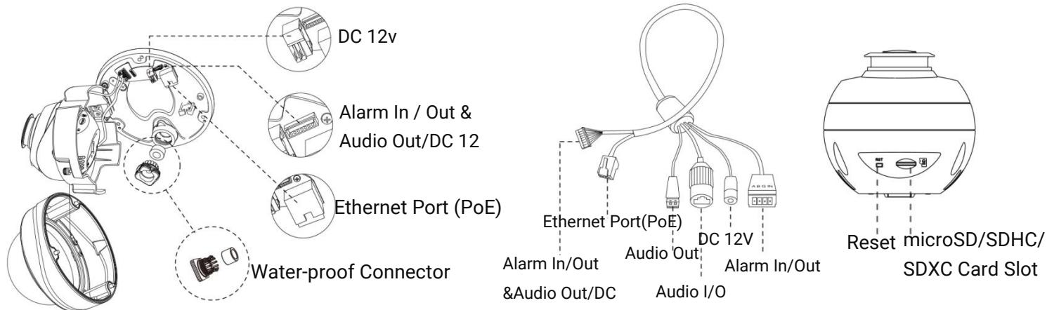
The cable is connected with the interface board by default.
